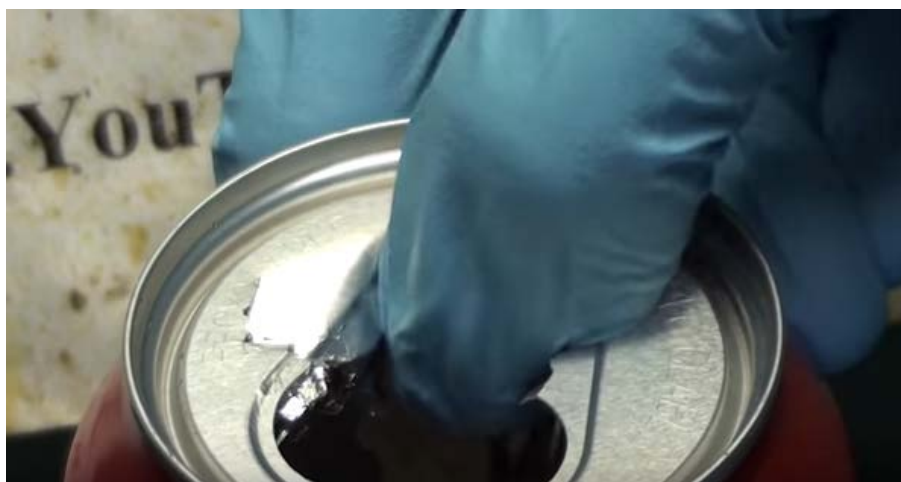
Figure 1. Liquid metal embrittlement by gallium metal on an aluminum soda can.
